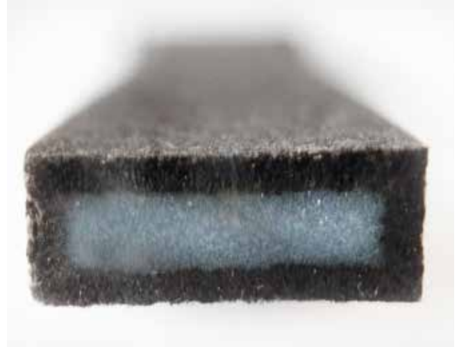
Fig. 4. Tensile test bar made from Akromid C3 GF 30 1 natural after 700 h at 210 °C (© Akro-Plastic)
